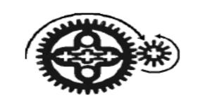
Gear ratio = <u>no of teeth on driven gear</u> no of teeth on driver gear
